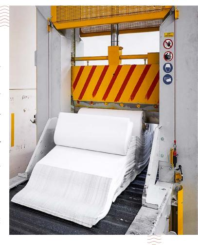
machines is not sent to the shredder but trans- ported in the other direction to the waste container. This high-quality material is re-used in stock preparation. And because the material is pre-shredded, it disintegrates in the pulper relatively quickly.
