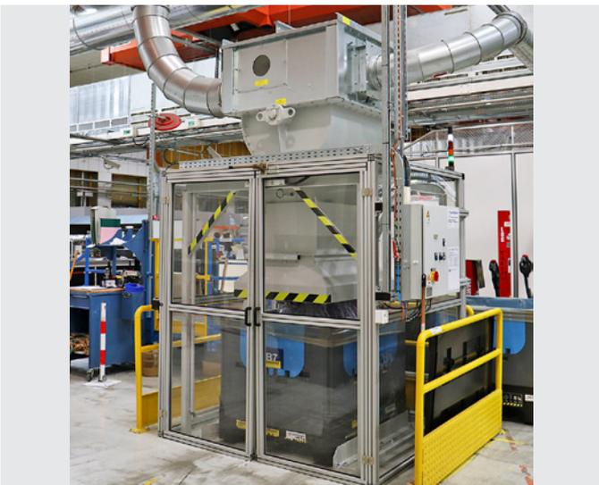
The margin strips are separated in a rotary cutter from the transport air and automatically compressed in a container.
