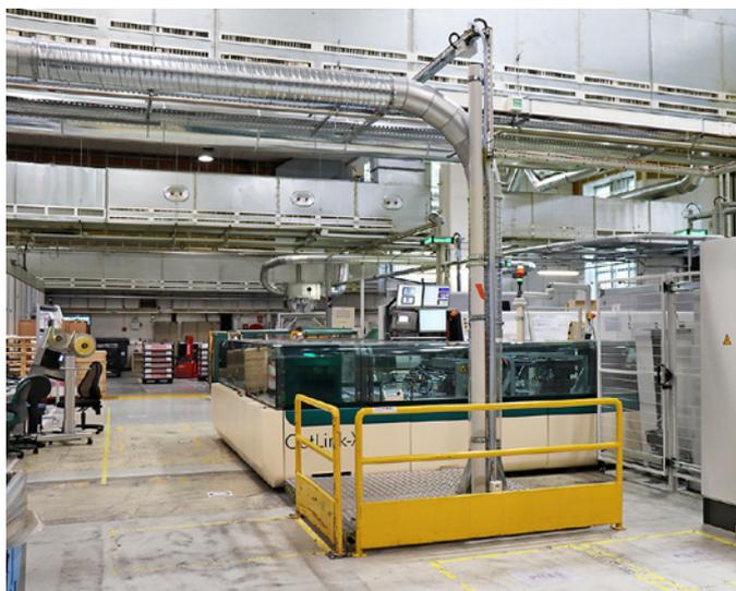
On each Cutlink-X-line, three suction positions are amalgamated to one duct.
