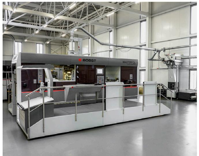
For the disposal of production waste from BOBST's foil embossing machines, Hunkeler Systeme AG developed a tailor-made suction technology.
