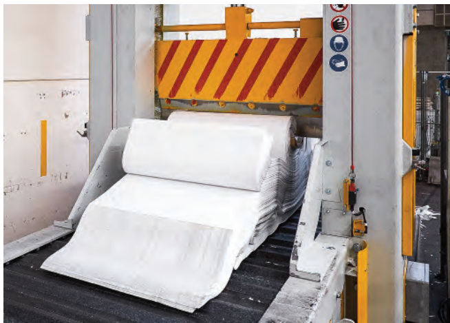
The splitting plant shreds substrate rolls in stacks whose width can vary between 20 and 80 centimeters.
