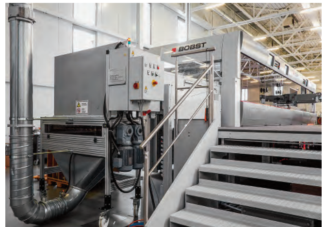
Currently, at the BOBST Competence Center in Mex, four die cutting machines are connected to a disposal system.
