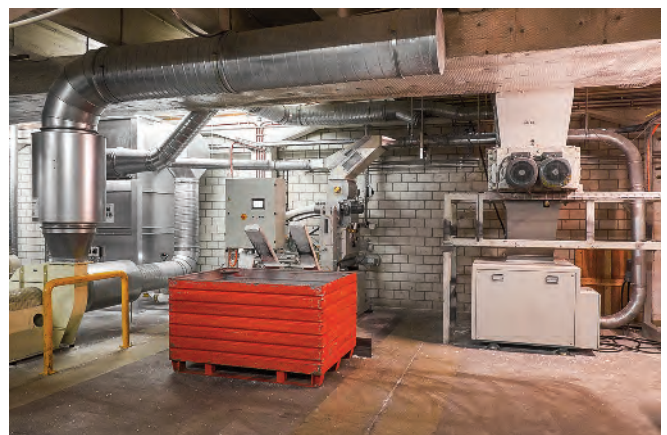
The end-product of the shredding process are small particles, which are compressed in a press (centre of picture) to briquettes.
