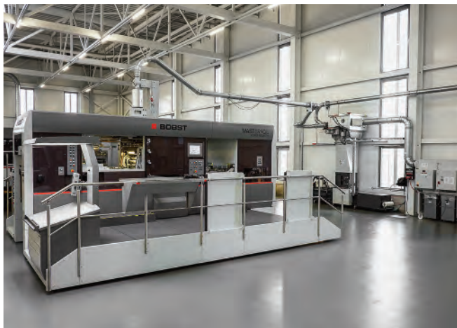
For the disposal of production waste from BOBST's foil embossing machines, Hunkeler Systeme AG developed a tailor-made suction technology.
