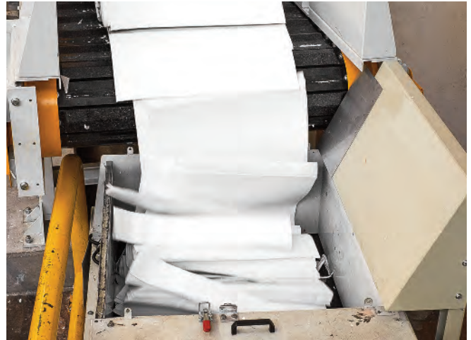
In a closed system, a conveyor belt transports the stack after the splitting process to a shredder with a downstream granulator.
