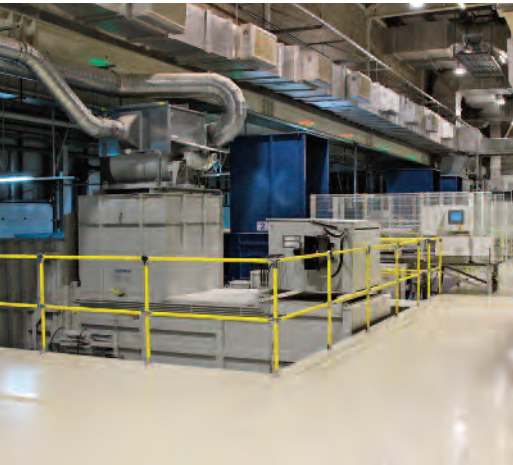
Al Nisr Publishing has fully automated the disposal of printing waste. No manual interference is necessary, from receiving the waste material at each production line to filling the container.
