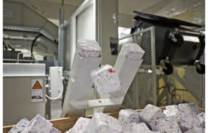
Simple, clean, secure: the shredded documents are compacted into briquettes with an edge length of 80×80×70 mm.
