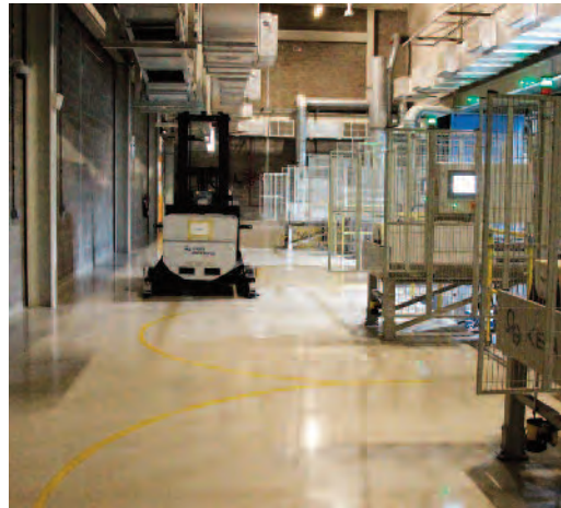
The disposal of rest rolls and roll sleeves, controlled by Laser Guided Vehicles, is in safe 'hands' thanks to an interface programmed by Hunkeler Systeme AG.
