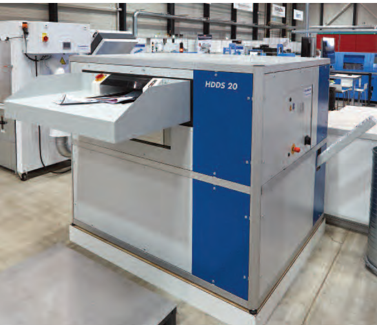
The new Document Destruction System HDDS 20 destroys paper in accordance with current security criteria.
