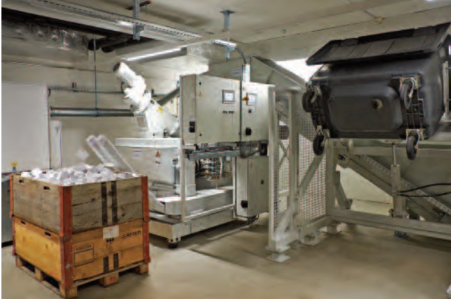
The shredding plant destroys confidential documentation in an Inline process – to security level P3 according to DIN 66399.
